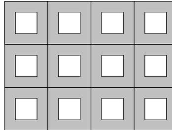
**FIGURE 3.** Periodic structure modelling the material (grey colour - carbonaceous matrix, white colour - Pd nanograins)
