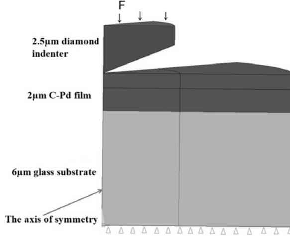
FIGURE 1. Axisymmetric model of the C-Pd film and indenter tip
