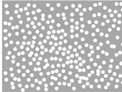
**FIGURE 2.** Schematic 2-d representation of the nanocomposite material (grey colour - carbonaceous matrix, white colour - Pd nanograins)
