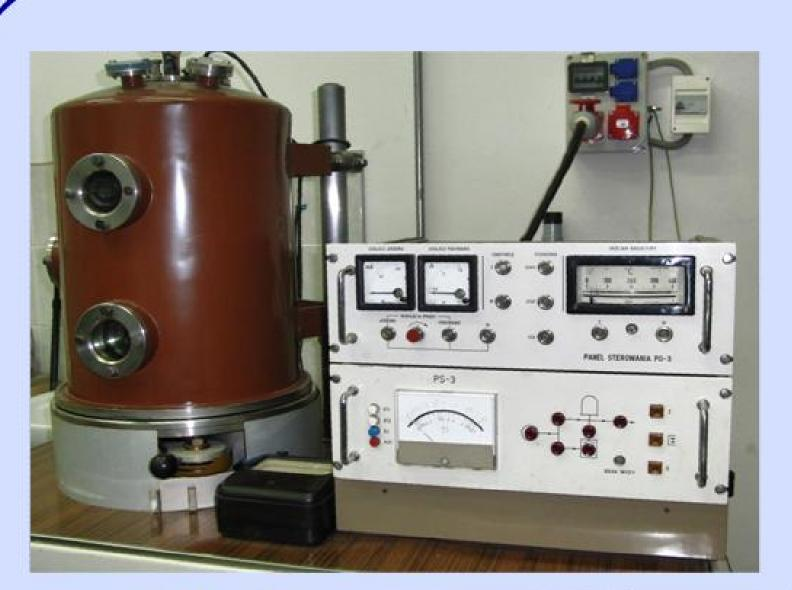
Fullerene C<sub>60</sub> and palladium acetate PdC<sub>2</sub>O<sub>4</sub> are precursors of the initial nanocomposite films in PVD process. Both compounds are evaporated at duration time t from two separated sources ( $C_{60}$  and  $PdC_2O_4$ ), at the distance d between sources and substrates.
