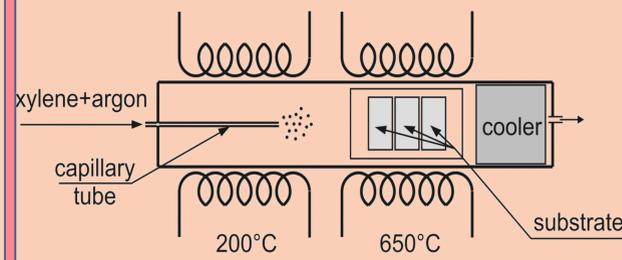
During CVD process carbon nanotubes films (2) grown by the decomposition of a hydrocarbon gas which was xylene. CVD process was performed in quartz tube in argon and xylene flow at 650 °C temperatures. In results we obtained films which consisted carbon nanotubes with different densities and sizes and also Ni nanoparticles placed on carbonaceous matrix or inside CNTs.
