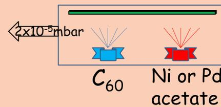
In PVD process two separated sources containing fullerene C<sub>60</sub> and nickel acetate or palladium acetate are used to prepare the initial films (1) and to cover by Pd the CVD film (3).
