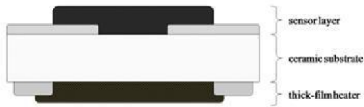
Fig. 1 Cross-section of the ceramic plate with the active film.
