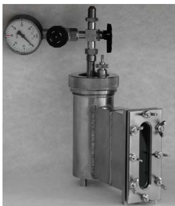
Fig. 1: Modified calorimetric bomb as a high-pressure reactor used for combustion synthesis.
