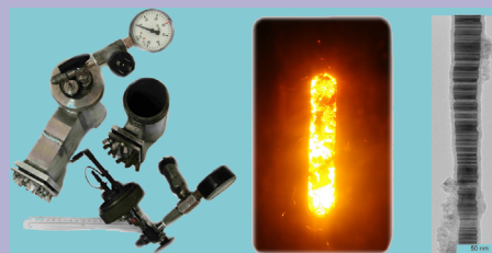
High-pressure reactor used for combustion synthesis, combustion reaction, and TEM of produced SiCNW
